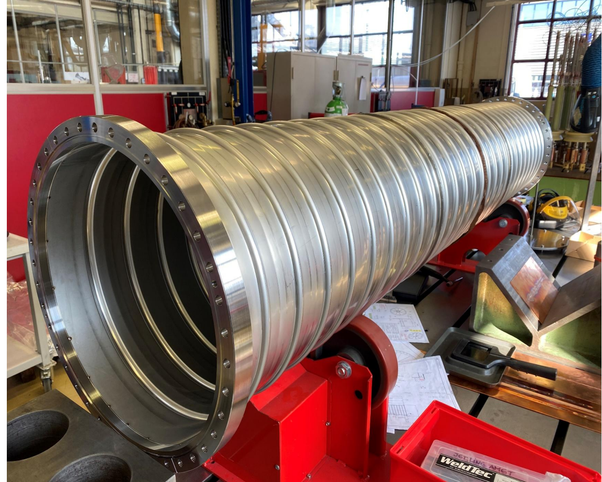
304L Pre-prototype available for UHV tests
